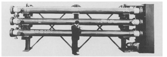
Scraped surface cooling crystallizers are well suited for use with sodium sulphate decahydrate (glauber's salt).
